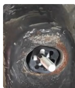
2 Install the plastic washer
