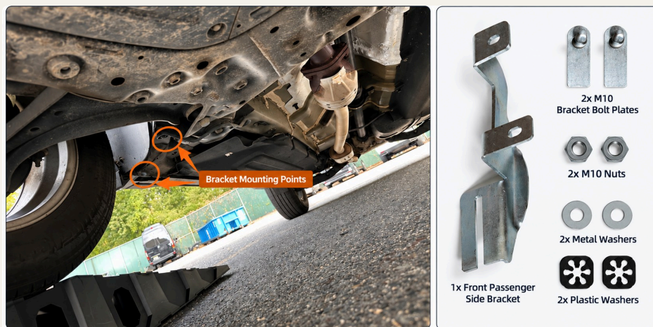
FRONT PASSENGER-SIDE BRACKET • MOUNTING POINTS & HARDWARE
