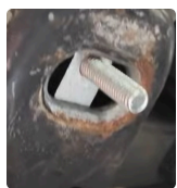
1 Insert the bolt plate
